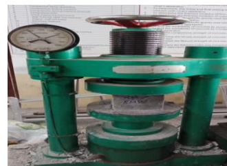
Fig. 6: Compressive strength testing of cube sample.
