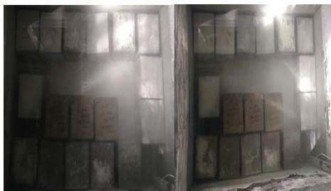
Fig. 5: Water curing of samples.
